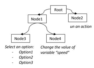
To reach our goal, any terminal node must have an associated user variable, in order to let the application (sketch code) be aware of the user interaction with the menu. This is done in MENWIZ binding a standard user variable to the terminal node: any change the user makes during menu interaction is available to the sketch code thru that variable and vice-versa (any change to the variable value done inside the sketch is available to the menu);
