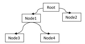
In the above image "Root" is the parent node of "Node1", and "Node1" is parent of "Node 3" and "Node 4".
