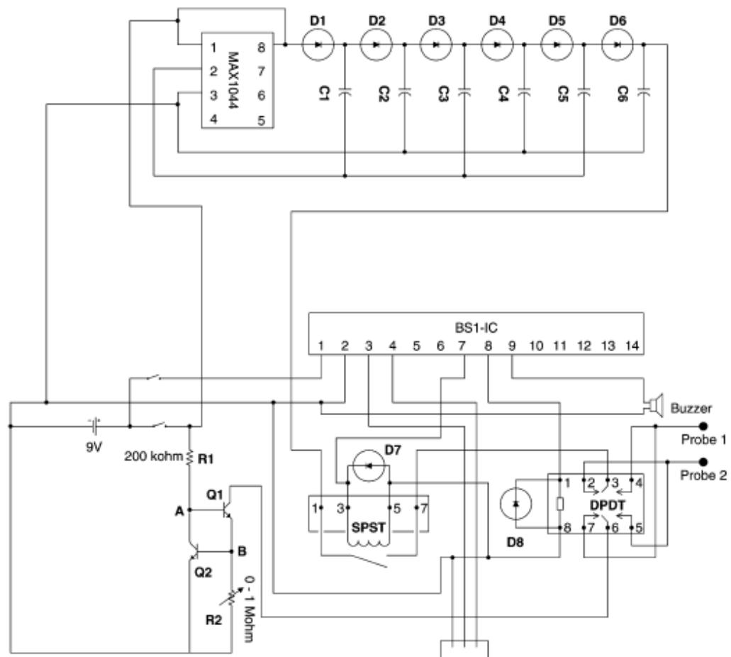
Fig. 1. Circuit diagram of the device. (a) Voltage booster, (b) constant current source and (c) current-waveform generator, where D1-D8 are 1N5817 diodes, C1-C6 are 10  $\mu$ F 35 V capacitors and Q1 and Q2 are 2N5550 transistors.
