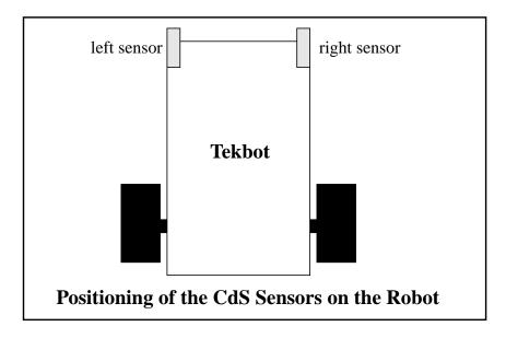
To understand the operation of the circuit, imagine that there is a CdS cell on each side of the robot. If the brightest area is directly in front of the robot, both cells are illuminated equally. This causes the voltage at the junction of the two cells to be 2.5 volts. This being the case, the upper and lower comparator's outputs will be at 5 volts causing both motors to go forward.
