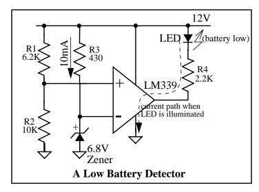
A reference voltage is established at the inverting input to the comparator by R3 and the 6.8 volt zener. R3 serves to limit the current through the 6.8 volt zener to about 10mA. The voltage developed across the zener is fairly stable over a wide range of zener current. To see why, go back and look at the steepness of the zener V-I curve in the reverse breakdown region.
