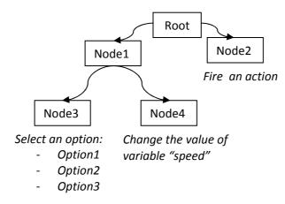
To reach our goal, any terminal node must have an associated user variable, in order to let the application (sketch code) be aware of the user interaction with the menu. This is done in MENWIZ binding a standard user variable to the terminal node: any change the user makes during menu interaction is available to the
