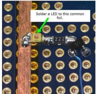
Other components can be soldered to the copper trace.
