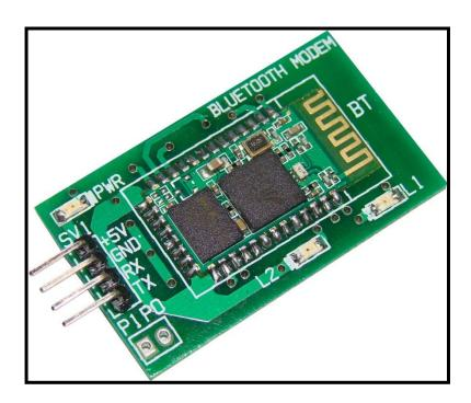
This Bluetooth modem is an easy to use module and can be directly interface to the microcontroller UART PINs, and specifically designed for transparent wireless serial connection setup. This design uses CSR's Bluetooth chips, V2.0 protocol standards with self-efficient on board antenna.
