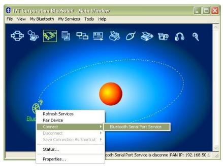
7. The connection is established and the software displays the COM Port where the Bluetooth is connected.
