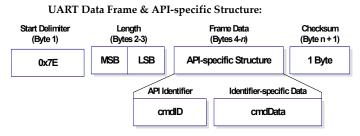
The cmdID frame (API-identifier) indicates which API messages will be contained in the cmdData frame (Identifier-specific data). Note that multi-byte values are sent big endian. The XBee modules support the following API frames:
