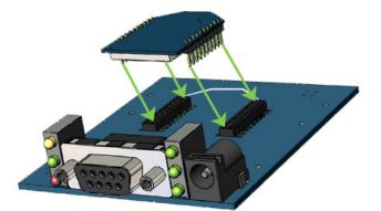
The receptacles used on Digi development boards are manufactured by Century Interconnect. Several other manufacturers provide comparable mounting solutions; however, Digi currently uses the following receptacles:
