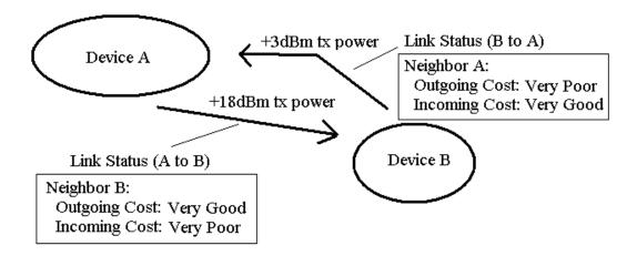
This mechanism enables devices A and B to recognize that the link is not reliable in both directions and select a different neighbor when establishing routes. (Such links are called asymmetric links, meaning the link quality is not similar in both directions.)
