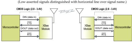
System Data Flow Diagram in a UART-interfaced environment (Low-asserted signals distinguished with horizontal line over signal name
