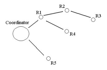
To send a source-routed packet to R3, the application must send a Create Source Route API frame (0x21) to the XBee, with a destination of R3, and 2 hops (R1 and R2). If the 64- bit address of R3 is 0x0013A200 404a1234 and the 16-bit addresses of R1, R2, and R3 are:
