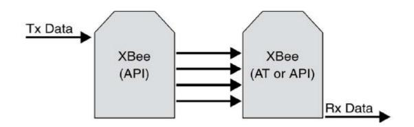
The API transmit frame can include up to 255 bytes of data, which will be broken up into multiple transmissions and reassembled on the receiving side. If one or more of the fragmented messages are not received by the receiving device, the receiver will drop the entire message, and the sender will indicate a transmission failure in the Tx Status API frame.
