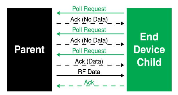
If the end device receives the acknowledgment and finds that the parent has no data for it, the end device can return to idle mode or sleep. Otherwise, it will remain awake to receive the data. This polling mechanism allows the end device to enter idle mode and turn its receiver off when RF data is not expected in order to reduce current consumption and conserve battery life.
