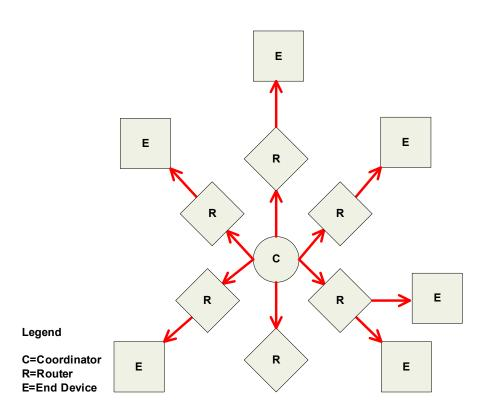
Each node that transmits the broadcast will also create an entry in a local broadcast transmission table. This entry is used to keep track of each received broadcast packet to ensure the packets are not endlessly transmitted. Each entry persists for 8 seconds. The broadcast transmission table holds 8 entries.
