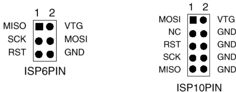
Figure 3-1. Standard ISP connectors on STK500, AVR ISP and STK200/STK300.
