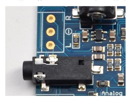
The headphone jack is a classic 3.5mm as seen in just about every audio device. You can connect this directly to any audio output. The terminal blocks are for if you have some direct-wiring project and you want a more permanent connection. You'll have to solder in the terminal
