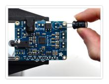
Capacitors are polarized, they have to be placed in the right way!
