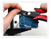
Clip down both of the long leads using diagonal cutters so they are nice and neat
