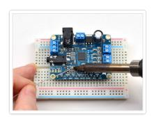
Finally, solder closed the **Analog** jumper on the left side.
