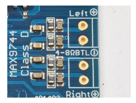
The speakers can be 4 to 8 ohm impedance, 20W maximum power. Since it is a class D amplifier, the signal out of these speaker blocks is a high frequency (~300KHz) PWM square wave. The inductance of the speaker smooths out this signal into audio frequencies of 20-20KHz.
