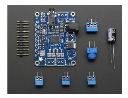
Each order comes with one MAX9744 breakout board with all surface-mount parts fully assembled and tested. We also include 3 x 2pin and 1 x 3pin terminal blocks, a 470uF power filter capacitor and  $1 \text{K}\Omega$  trim pot. To use this board, a little soldering is required to attach the terminal blocks and other components, but its fairly easy and expect it should take less than 15 minutes.
