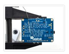
Flip over the board so you can solder the two pads
