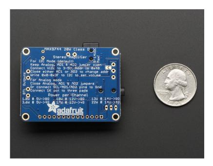
We like the MAX9744 amplifier at the heart of this board because its very easy to use, but it also has both analog and digital volume control capability. Use a single  $1K\Omega$  pot (we include
