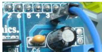
Above: original Adafruit Motorshield with Pi2 “wired/connected/ to hole Below: Clone with blue cable welded on the hole
