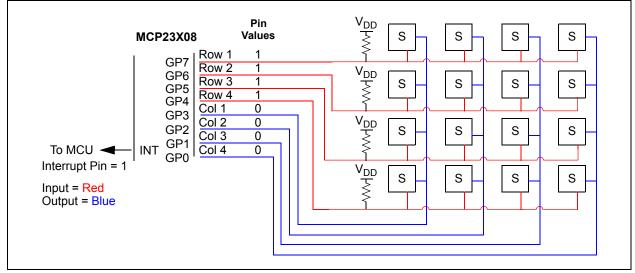
FIGURE 3: Initial Setup.
