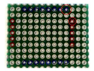
The "ESP" side again, with component labels. The horizontal rows are for the ESP8266. The vertical rows are for the MAX module.
