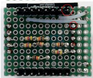
The next step is to solder the ESP board to the header pins prepared for it. Again, ensure the correct orientation!
