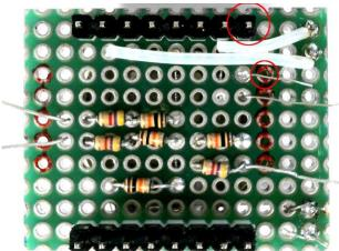
The "MAX" side of the board flipped along a vertical axis showing the connections. Refer to the schematic if a connection is not clear from this picture.
