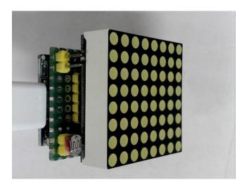
It uses a Wemos D1 Mini pattern ESP8266 micro controller and a Robotdyn 8x8 led module with a Max 7221 driver chip.
