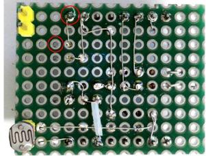
The MAX module has now been soldered in and 5 connections made to it. Ensure the correct orientation!
