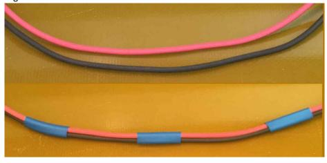
15. Insulate series resistors, diodes etc.
