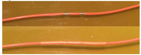
18. Strain relief for cable connectors.
