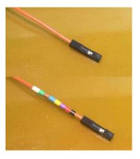
5. Water proofing splice joints.
