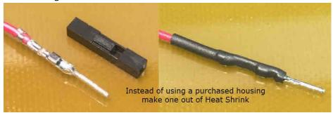
17. Repair damaged wires.
