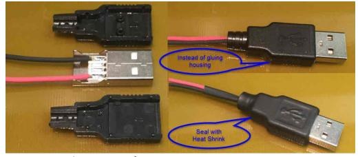
10. Lock connectors together, cut apart if necessary.
