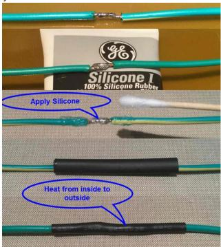
6. Building up the diameter of a cable to fit an opening.
