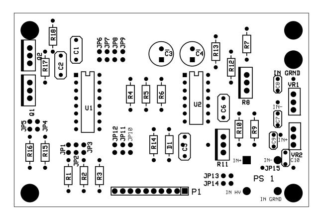
Component location and board layout for the INA125 Amplifier Module.
