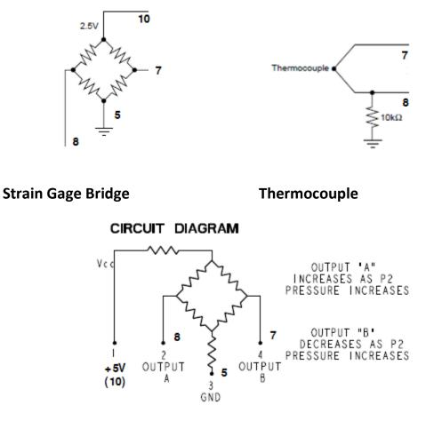
Honeywell Pressure Transducer (26PC Series)
